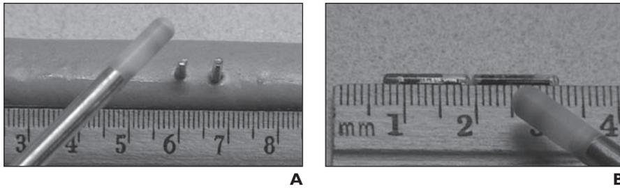
**Fig. 6**—Photographs show pencil-probe radiofrequency identification (RFID) reader attachment (TagFinder, Health Beacons) approaching RFID tags. Scale is millimeters.
