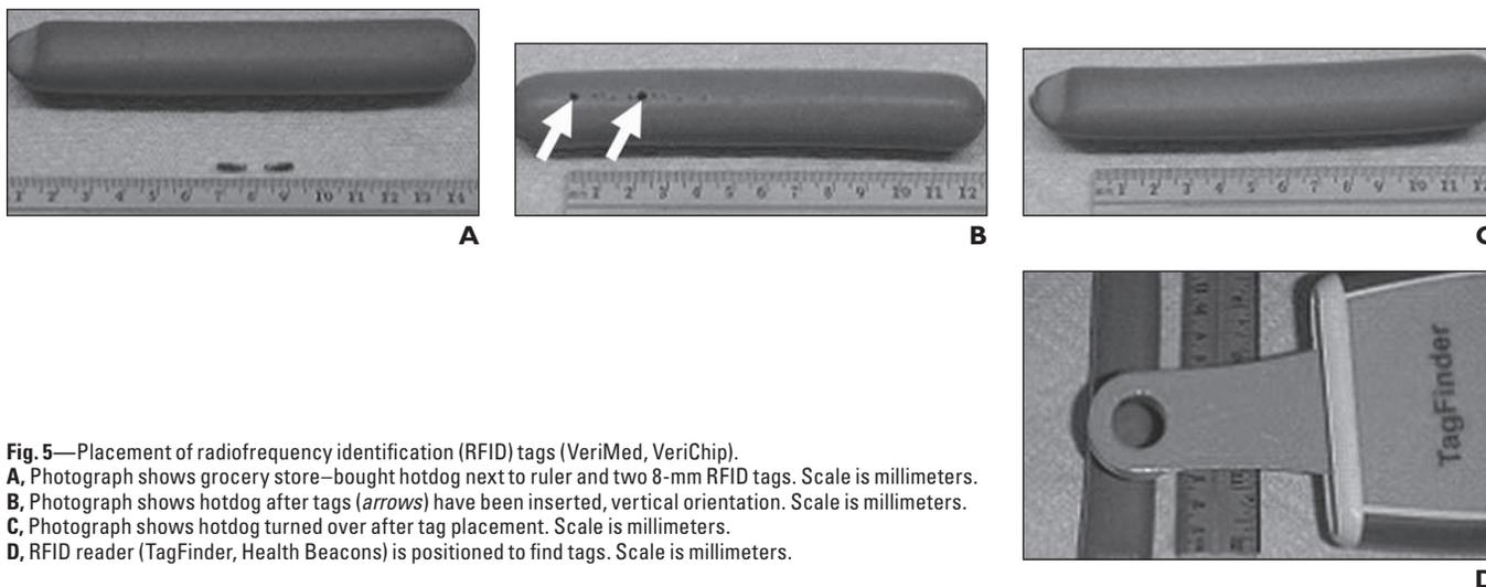
**Fig. 5**—Placement of radiofrequency identification (RFID) tags (VeriMed, VeriChip). **A**, Photograph shows grocery store-bought hotdog next to ruler and two 8-mm RFID tags. Scale is millimeters. **B**, Photograph shows hotdog after tags (arrows) have been inserted, vertical orientation. Scale is millimeters. **C**, Photograph shows hotdog turned over after tag placement. Scale is millimeters. **D**, RFID reader (TagFinder, Health Beacons) is positioned to find tags. Scale is millimeters.
