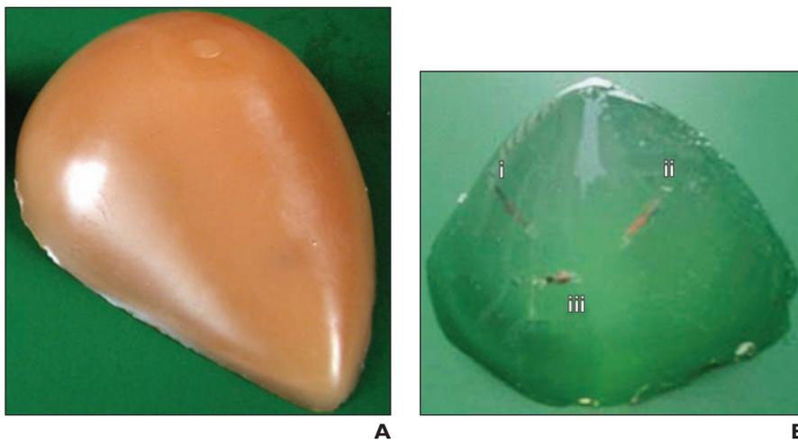
**Fig. 4**—Breast phantoms used for radiofrequency identification (RFID) tag depth detection testing. **A**, Opaque sonography breast phantom. **B**, Gelatin with implanted RFID tags at insertion depths of 2 cm (i), 3 cm (ii), and 1 cm (iii).
