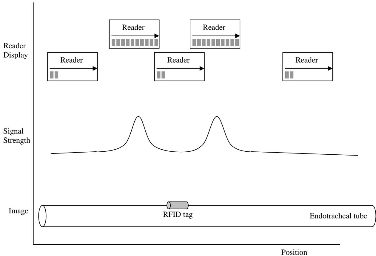
Fig. 2. The RFID reader shows signal peaks when adjacent to the longitudinal ends of the tag.
